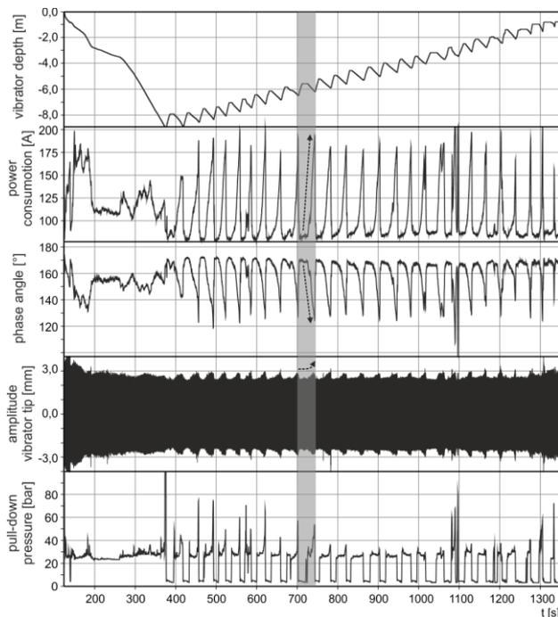
Figure 4. Time history of the vibrator depth, current power consumption of the electric engine, amplitude of the vibrator tip, phase angle, pull-down pressure during deep vibro compaction in standard operation mode.
