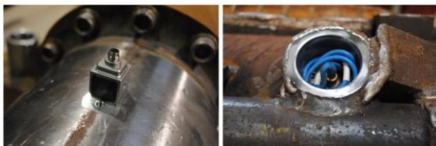
Figure 3. Triaxial accelerometer on the vibrator body (left), sensor installation in steel cylinders (right).
