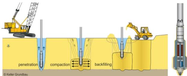
Figure 1. Compaction process during deep vibro compaction and the deep vibrator.
