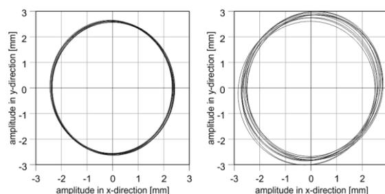
Figure 5. Horizontal movement of the vibrator tip at the beginning (left) and at the end (right) of the lowering process during the highlighted pilgrim step.
