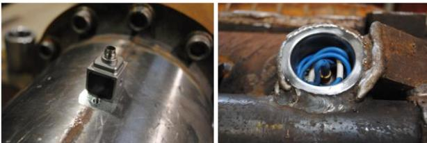
Figure 6. Triaxial accelerometer on the vibrator body (left), sensor installation in steel cylinders (right).
