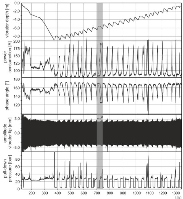
Figure 8. Time history of the vibrator depth, current power consumption of the electric engine, amplitude of the vibrator tip, phase angle, pull-down pressure during deep vibro compaction in standard operation mode.
