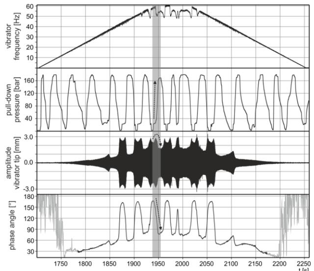
Figure 10. Time history of the vibrator frequency, pull down pressure, amplitude of the vibrator tip and phase angle, during a test with non-standard process parameters.
