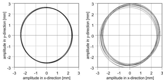
Figure 9. Horizontal movement of the vibrator tip at the beginning (left) and at the end (right) of the lowering process during the highlighted pilgrim step.
