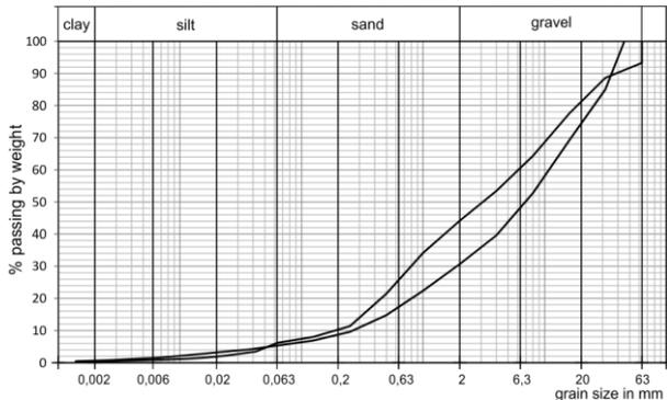
Figure 5. Grain size distribution curves of the subsoil on the test area.
