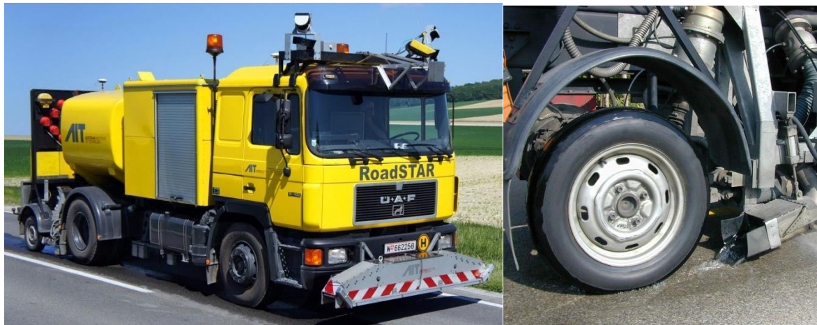
1 2 3 FIGURE 1 Monitoring device RoadSTAR (left); detail of the skid resistance measurement 4 unit (right)
