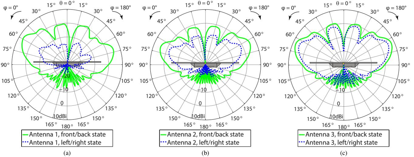
Fig. 6. Measured vertical cuts of the gain patterns at 2.45 GHz for azimuth  $\varphi = 0^\circ$  of a) antenna 1, b) antenna 2 and c) antenna 3. If the cavity is mounted on the vehicle according to Fig. 1, the  $\varphi = 0^\circ$  coincides with driving direction and  $\varphi = 180^\circ$  are the patterns towards the rear of the vehicle.
