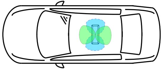
Fig. 1. A pattern reconfigurable antenna is concealed inside a chassis antenna module. Exemplary mounting location on a car roof.
