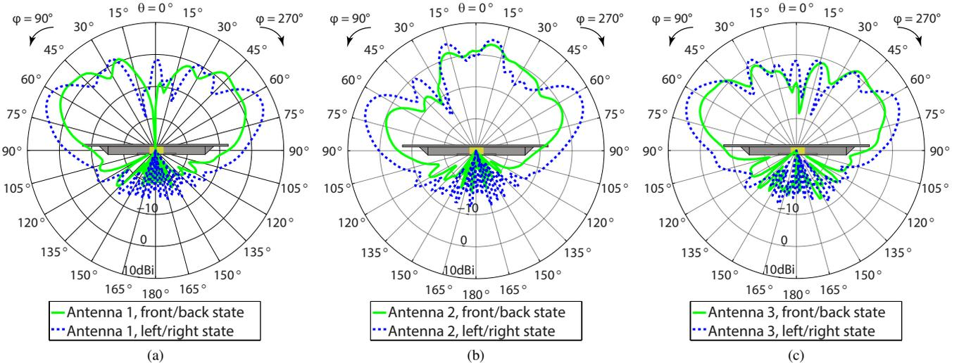
Fig. 7. Measured vertical cuts of the gain patterns at 2.45 GHz for azimuth  $\varphi = 90^\circ$  of a) antenna 1, b) antenna 2 and c) antenna 3. If the cavity is mounted on the vehicle according to Fig. 1, these cuts coincide with the left and right side of the vehicle.
