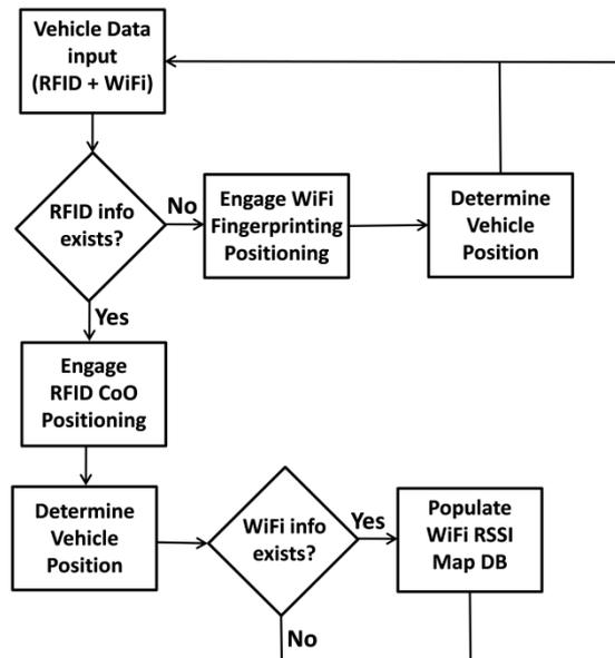
Figure 8: Flowchart of the proposed localization scheme with the simultaneous dynamic radio map updating
