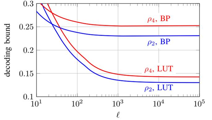
Fig. 2: Decoding bound convergence for BP and 4-bit LUT decoding and two CN degree distributions from Table I in a BI-AWGN channel with  $\sigma = 0.929$ .
