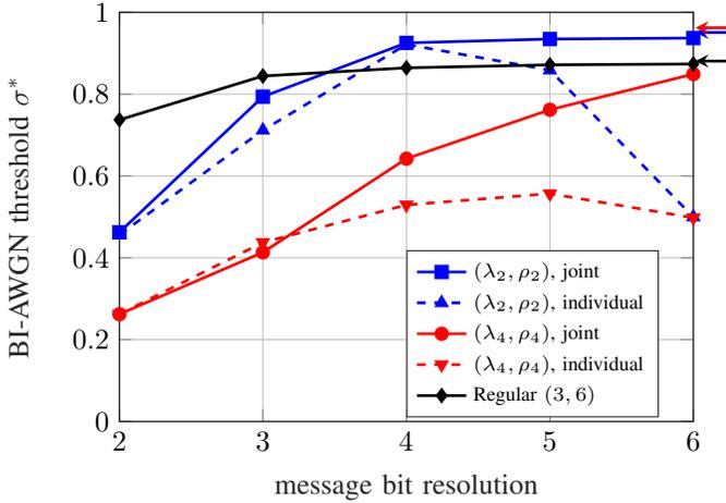
Fig. 1: DE thresholds versus message resolution for different LDPC ensembles in a BI-AWGN channel with individual and joint LUT design. Arrows on the right margin indicate the corresponding BP thresholds.
