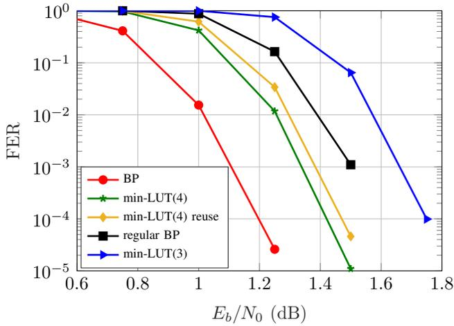
Fig. 3: FER Simulations for different codes of length  $N = 10000$  and 100 decoding iterations
