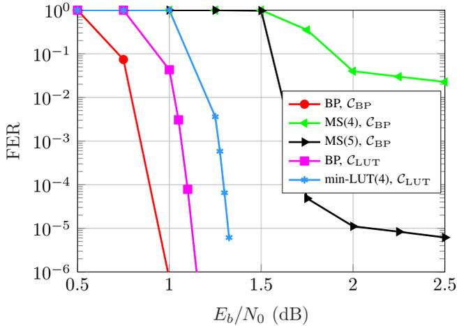
Fig. 4: FER Simulations for the LUT optimized code  $C_{LUT}$  and the BP optimized DVB-S2 code  $C_{BP}$ . For for both codes  $N = 64800$  and for all decoders 100 decoding iterations have been performed.
