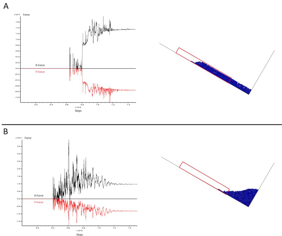
Figure 4: Impact force vs. calculation steps (left) and end position of the released blocks (right) for a runout distance of 50 m and a block volume of 1 m<sup>3</sup>. The red rectangle indicates the release position of the simulated 1000 rock blocks. A) rotational velocity fixed, B) rotational velocity free
