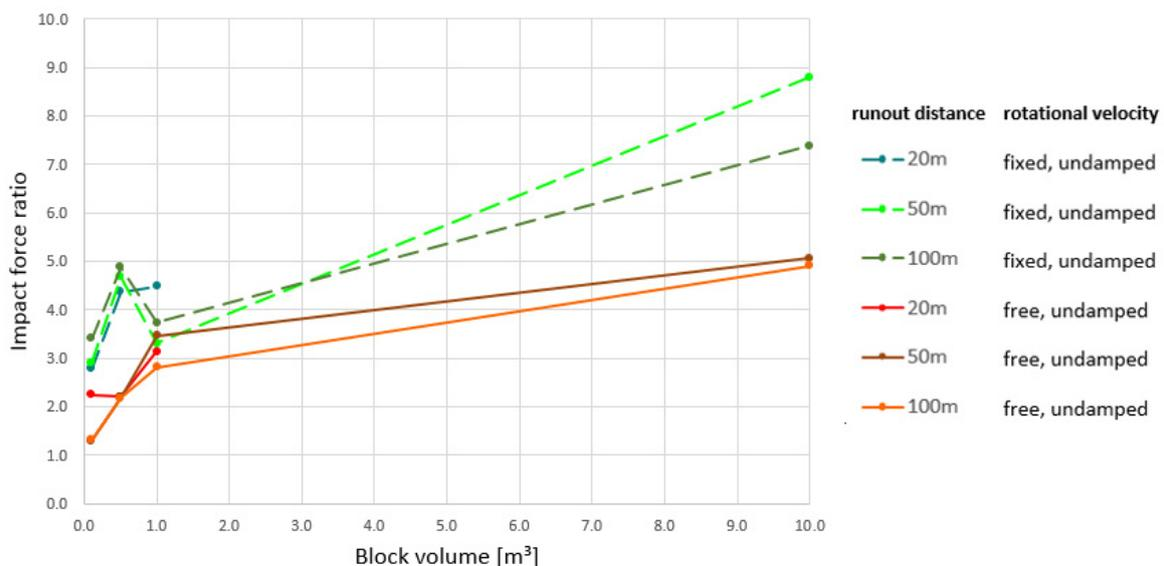
Figure 3: Ratio of the maximum impact force generated by single rock fall and rock mass fall (impact force ratio) for single block volumes of 0.1, 0.5, 1.0 and 10.0 m<sup>3</sup>.
