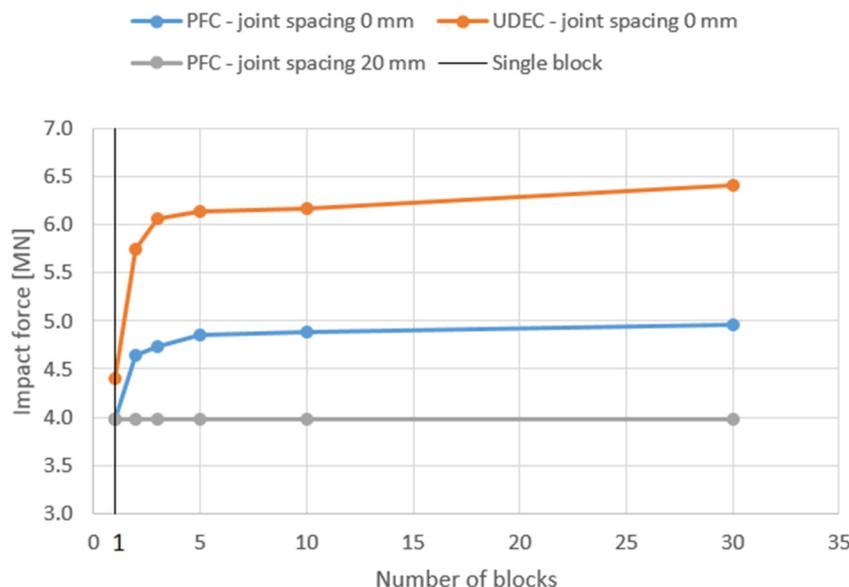
Figure 2: Maximum impact force vs number of blocks
