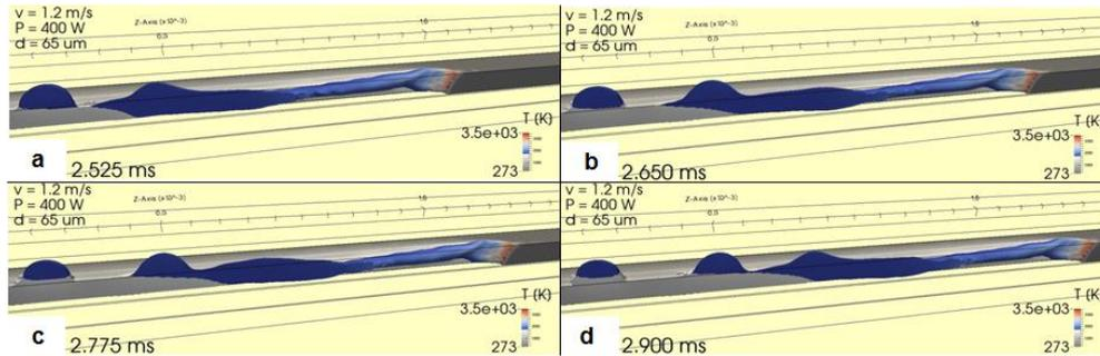
Fig. 4 Different stages of the hump formation in the course of the micro welding process.
