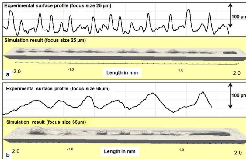
Fig. 5 Comparison between simulation results and experimental ones with the spot size of 25  $\mu\text{m}$  and 65  $\mu\text{m}$ , respectively.
