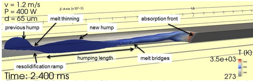
Fig. 3 Schematic view of the process showing the most relevant areas involved.
