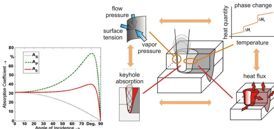
Fig. 1. Schematic summary of the simulation model.
