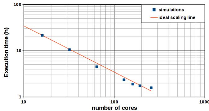
Fig. 6. Simulation performance in parallel for a benchmark case with a fixed grid of about 4 million of elements. The red line indicates the ideal trend where the simulation time decreases linearly with the number of cores used. The beginning of the stagnation area shows up at a level of exactly 20 thousand cells per core when using 192 cores.
