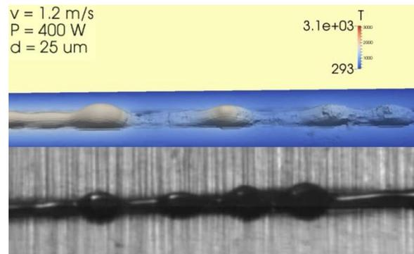
Fig. 2. Hump structures given by the simulations as well as by the experimental test with the spot size of 25  $\mu\text{m}$ .
