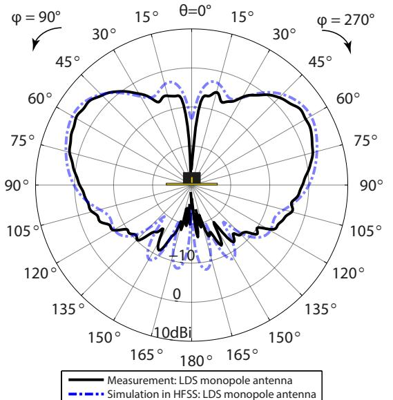
Fig. 3: Gain pattern of the LDS monopole antenna for 5.9 GHz without the cavity on a small  $150 \times 150 \text{ mm}^2$  ground plane.
