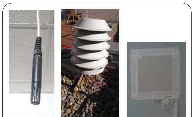
Figure 5: Left: The Lin Picco sensor inside (protected by a plastic cover). Middle: Lin Picco sensor exterior protected by protective shield. Right: Heat flux film.
