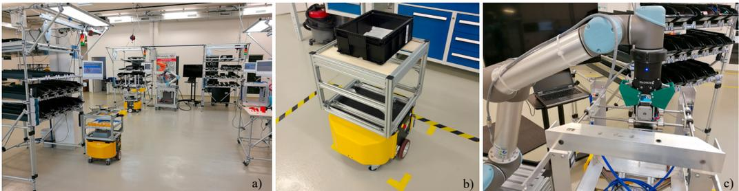
Fig. 2: a) Assembly line in PFI40 with AGV in front (yellow) and handling robot (blue) in the background, b) Autonomous vehicle for materials transport, c) Single arm robot assists human in the mounting tasks.
