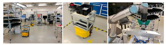
Fig. 2: a) Assembly line in PFI40 with AGV in front (yellow) and handling robot (blue) in the background, b) Autonomous vehicle for materials transport, c) Single arm robot assists human in the mounting tasks.
