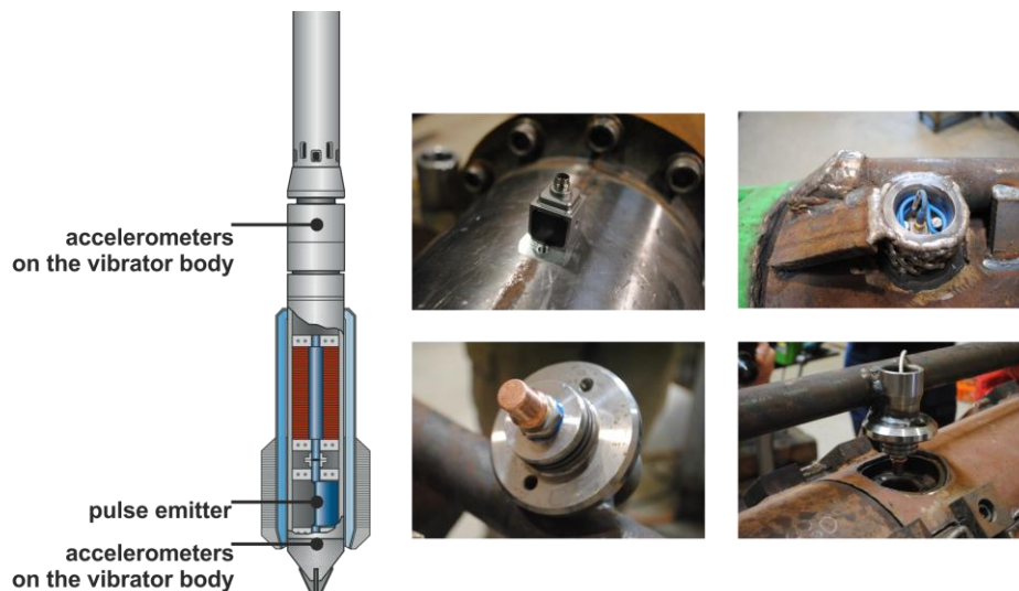
Figure 3. The position of the triaxial accelerometers and the pulse emitter on the vibrator body (left), installation of the accelerometers and the of the pulse emitter in the vibrator body (right).
