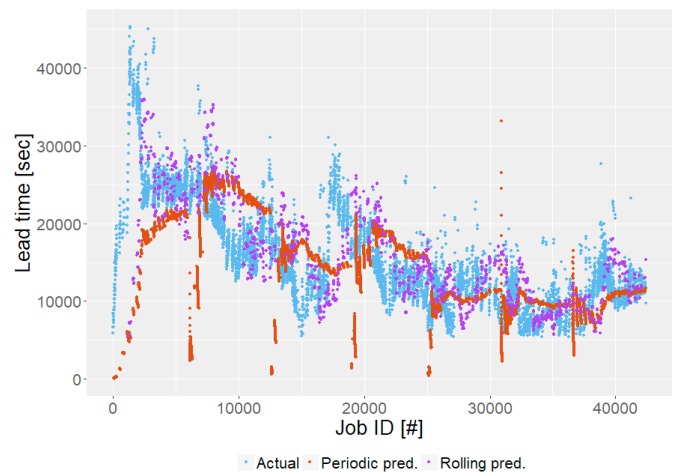
Fig. 2. Job lead times with finite interval Little’s law (job type A): actual LT values, one-day periodic and one-day rolling horizon prediction
