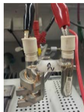
Figure 2 Electrolytic crystallization of the networks
