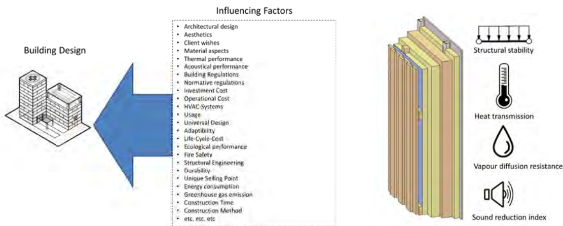
Figure 1: (left) Influencing parameters on building design; (right) Important aspects that need to be considered in the design of an exterior wall
