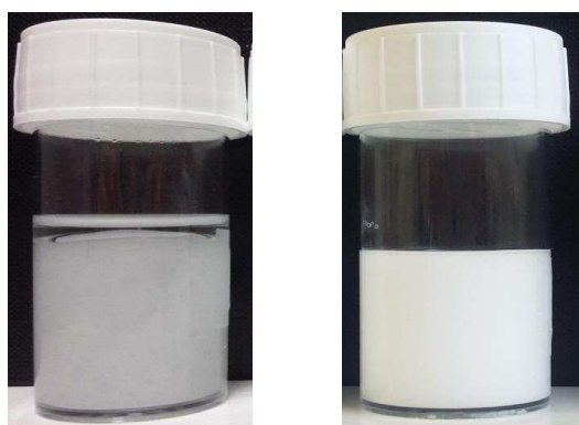
Figure 1. Photographs of oil-in-water emulsions containing pristine xanthan one day after preparation (left) and containing modified xanthan after 3 months (right).
