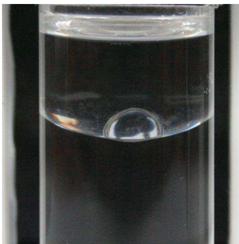
Figure 1. A water droplet stabilized on the interface between toluene (upper phase) and water (lower phase). Stabilization is achieved by dispersing a lamellar compound in the organic phase.
