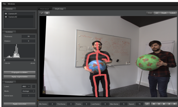
Fig. 4. User interface of the post-correction tool with scribble placed by the user on a key-frame. The histogram displayed on the left shows the disparities covered by the scribble and supports the segmentation of the selected object and projection of the scribble to other views.
