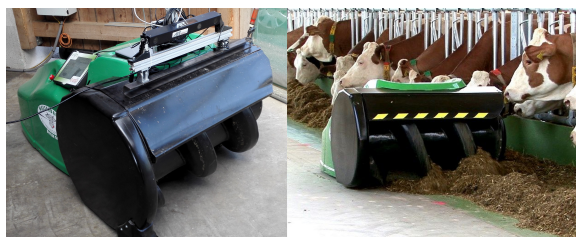
Fig. 1: Target robot platform for feeding with front-facing stereo camera system. Right image: © Wasserbauer
