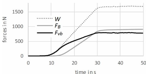
**Figure 6. Distribution of the bulk weight on bunker and belt**
