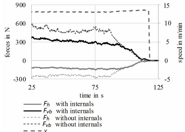
Figure 11. Emptying forces with and without internals at an outlet height of 30 mm
