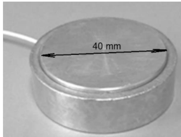
**Figure 4. Pressure sensor for direct measurement of the vertical stress acting on the belt**
