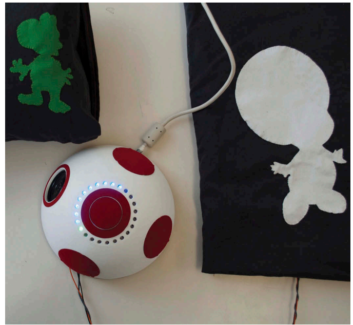
Figure 13. The rattle alarm system – Developed together with Mia – left: cushion, middle: alarm clock, right: pressure mat.
