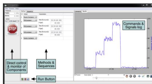
Figure 2: Instrumentino user interface (GUI) to control and monitor CE experiments (reprinted with permission from I.J. Koenka)
