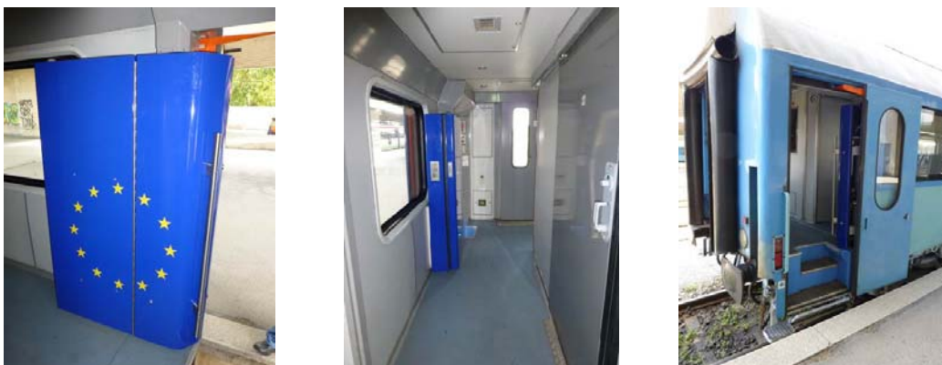
Fig 1.: BAS in the stored position installed in a UIC-vehicle (from BDZ - Bulgaria)
