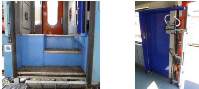
Fig 2.: Assembly point for the BAS
