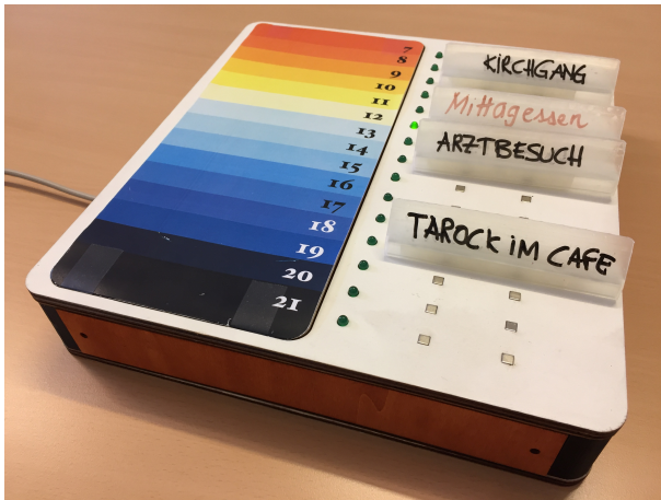
Fig. 1. This Figure shows the first haptic prototype of the day planner. The left side shows the time of day. Blocks can be placed on the right side and are labelled with activities. A glowing LED shows the current time of the day.
