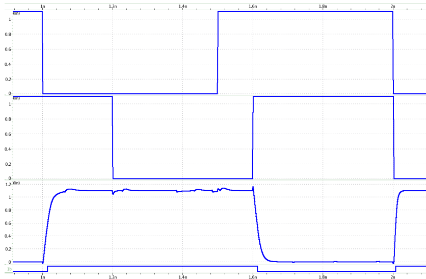
Figure 4.4: Switching waveforms for a NAND gate.
