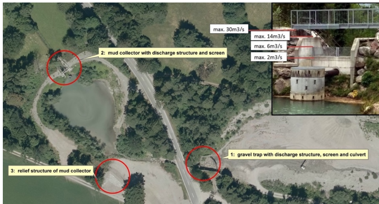
Figure 54: Detailed overview of the different technical structures in a torrent (Office for Civil Protection ©)
