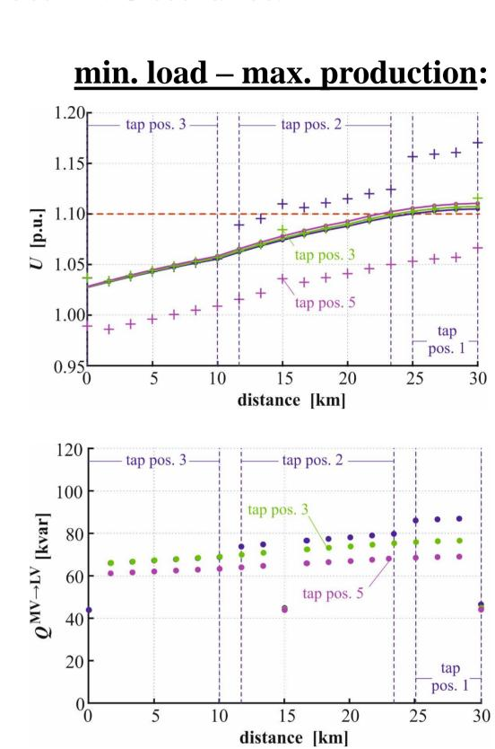
Results show that in the case of uncontrolled PV-systems the DTRs' tap positions have a slight impact on MVG's voltage profile and on the *Q*-consumption of LVGs. Increasing the DTRs' tap positions decreases LVG voltages and thus the *Q*-consumption of ZIP-loads. This slightly increases MVG voltages.
