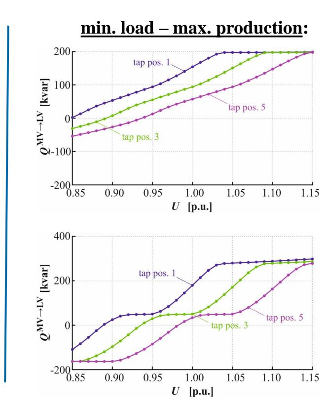
Results show that the DTRs' tap positions have a strong impact on the LVGs' Q(U)-characteristics, if PV-systems are Q(U)-controlled. Increasing the DTRs' tap positions shifts the characteristic to the right.
