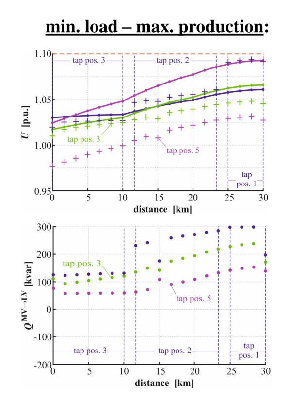
Results show that in the case of Q(U)-controlled PV-systems, the DTRs' tap positions have a strong impact on MVG's voltage profile and on the Q-consumption of LVGs. Increasing the DTRs' tap positions decreases LVG voltages and thus the Q-consumption of ZIP-loads and PV-systems. In return, this significantly increases the voltages in MVG.
