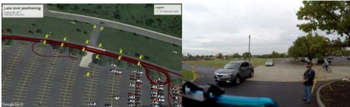
Figure 6: Lane level experiment. On the left: map of the trajectory for 1 car. On the right: a photograph of the data collection process and the experimental set-up on field.
