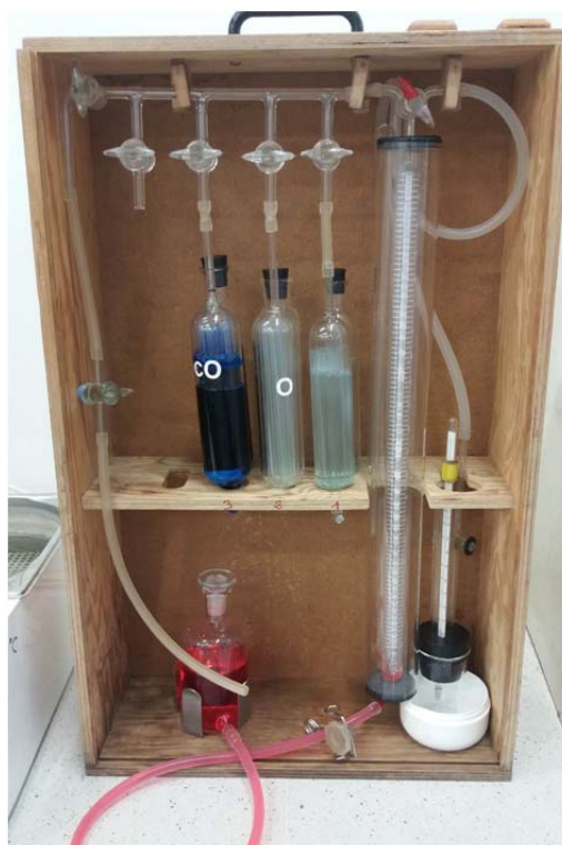
Figure 1: Örsat gas analyzer used during the research
