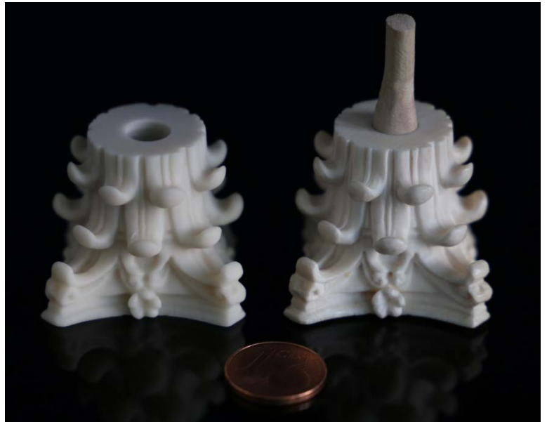
Figure 2: Comparison of the manufactured (left) and the original (right) column capital of the cabinet of king Friederick the Fair.
