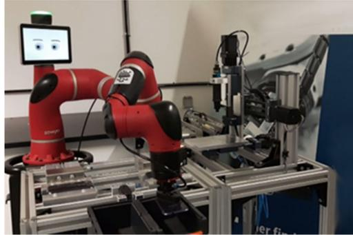
Figure 1: Disassembly machinery demonstrator with Sawyer-Robot. Source: sustainablySMART
