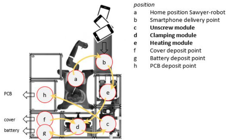
Figure 4: Basic scenario, necessary movements for mobile phone disassembly scenario
