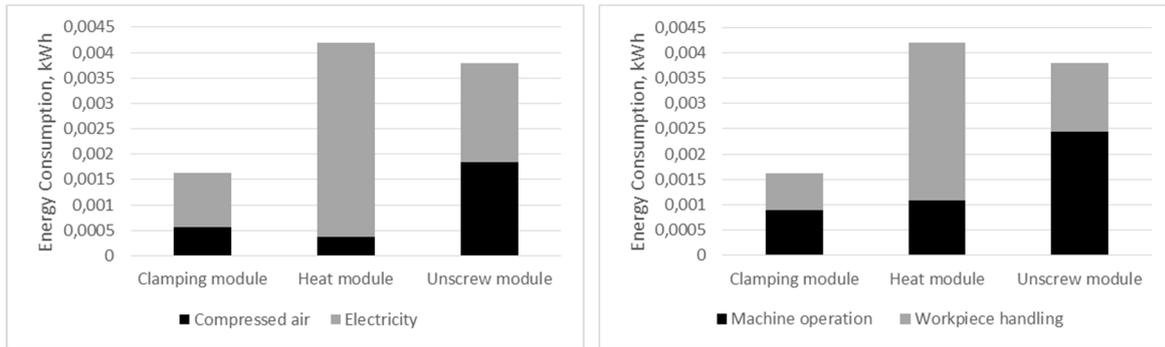
Figure 6: Energy consumption of modules processing one phone. Left: Types of energy / Right: Machine tool functions
