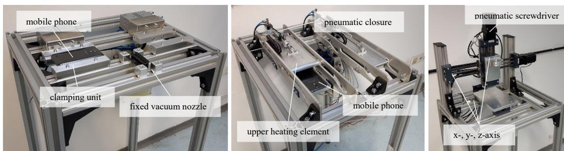
Figure 2: Dismantling Modules for a flexible mobile phone disassembly process: Clamping Module / Heating Module / Unscrew Module. Source: ProAutomation
