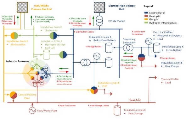
Figure 1: Topology of the optimization model for an urban energy system
