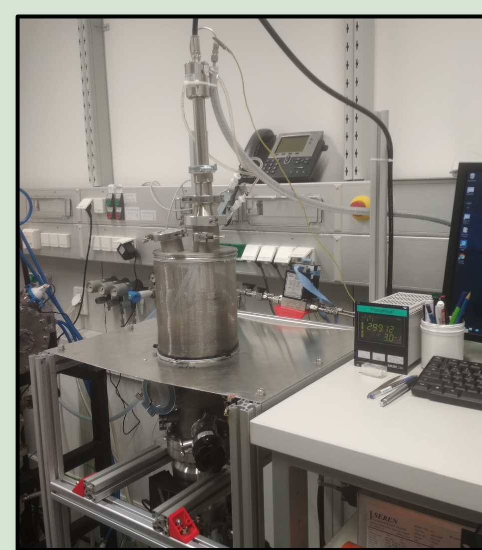
The device for RF-sputtering was built in-house. Alongside Ar, reactive gases ( \text{O}_2 and \text{N}_2 ) can be introduced. Wires inside the chamber allow for electrochemical measurements without opening the chamber.
