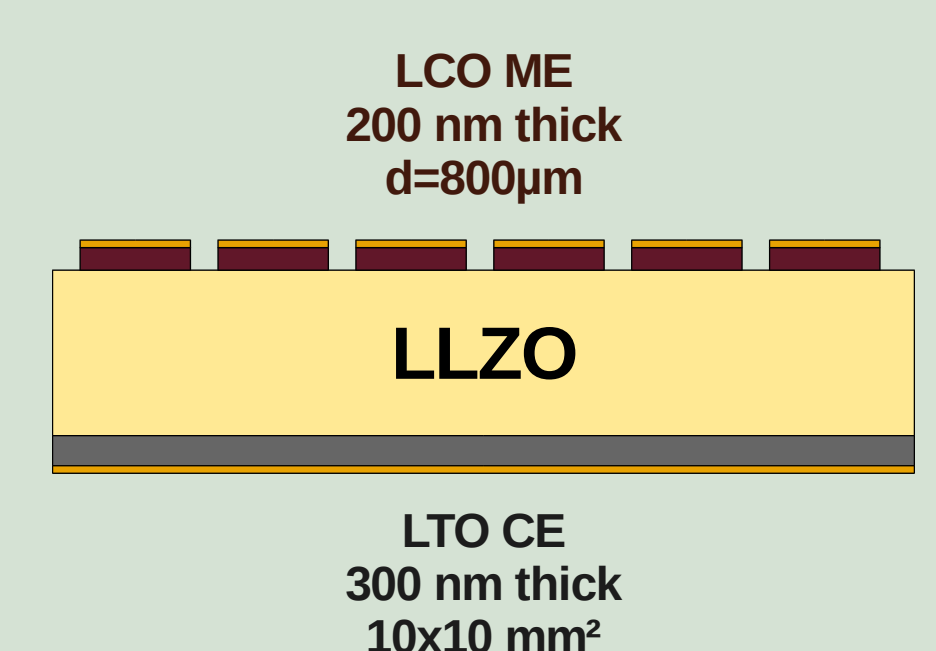
Schematic of an all solid state cell which was prepared by sputtering LTO and LCO onto a Ta:LLZO single crystal. The sample was annealed twice to achieve crystalline electrode materials.
