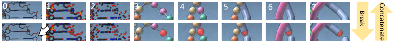
Fig. 5: Breaking & concatenating single strands, in multiple scales. After changes are done in one scale, we propagate the effects to other scales. Breaking a single strand does not break the double strand, thus Scales 8 and 9 are not visually affected.
