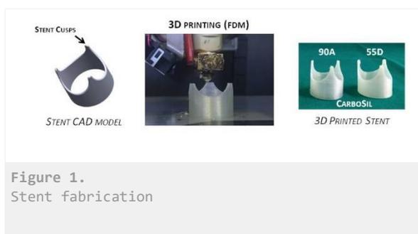
Figure 1. Stent fabrication
