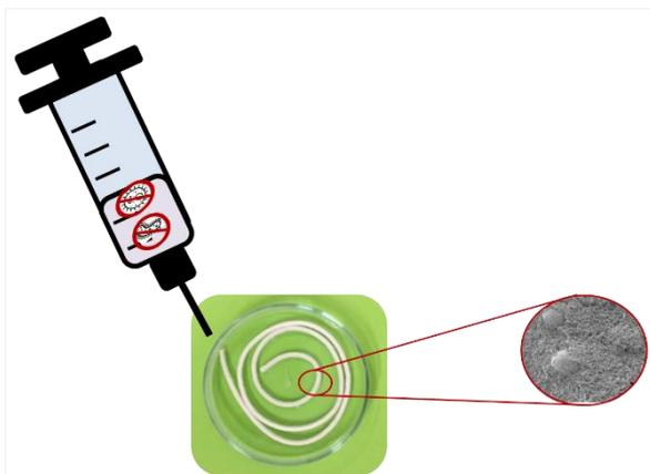
**Cement wire extruded in saline solution.**
