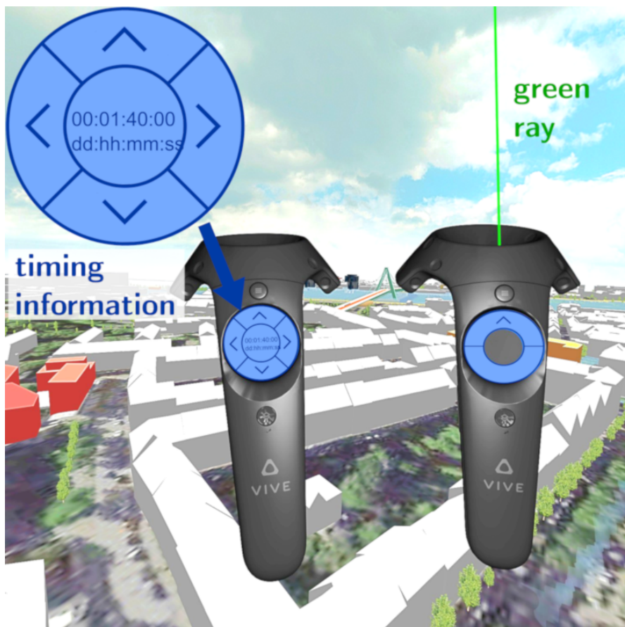
Figure 4.1: Screen shots of the controllers in the VE, extended by annotations. The left controller is the so called mode controller, the right one is the steering controller.
