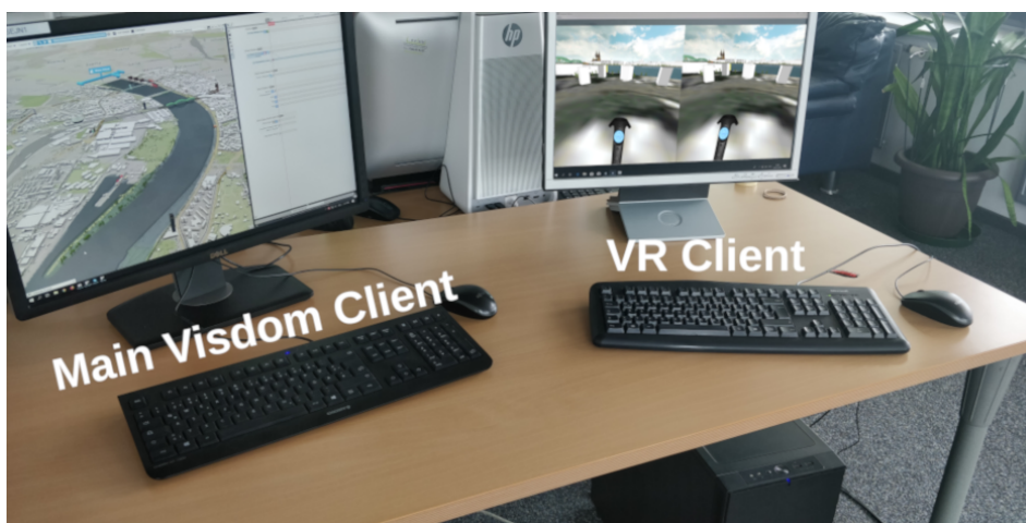
Figure 3.5: Basic Operator-Trainee setup. The operator-PC runs the Visdom Client and the other PC is responsible for running the VR application. Image has been taken by the author.
