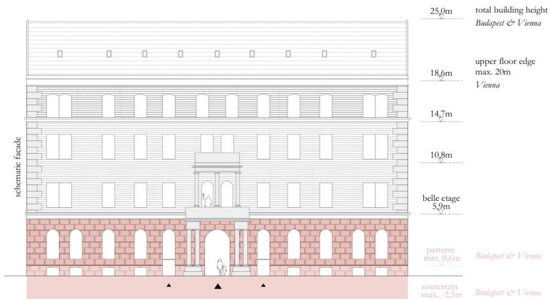
Figure 3. Schematic elevation of the Gründerzeit building typology
