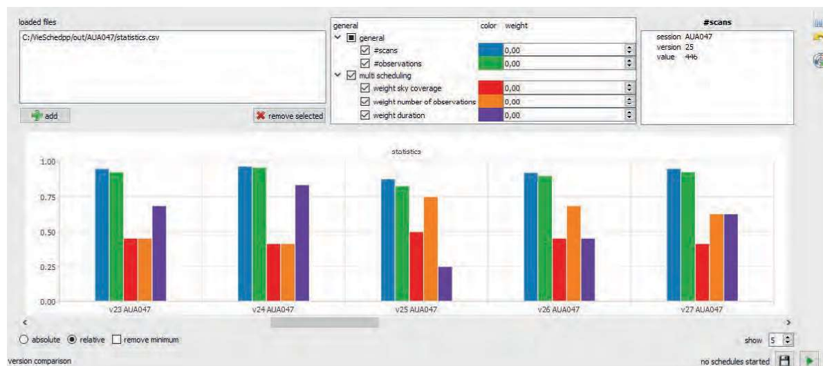
Fig. 2: VieSched++ statistics tool for comparing created schedules using the multi-scheduling tool. The bars symbolise the relative value of parameters such as, number of scans (blue), number of observations (green) and weight factors (red, orange, purple).
