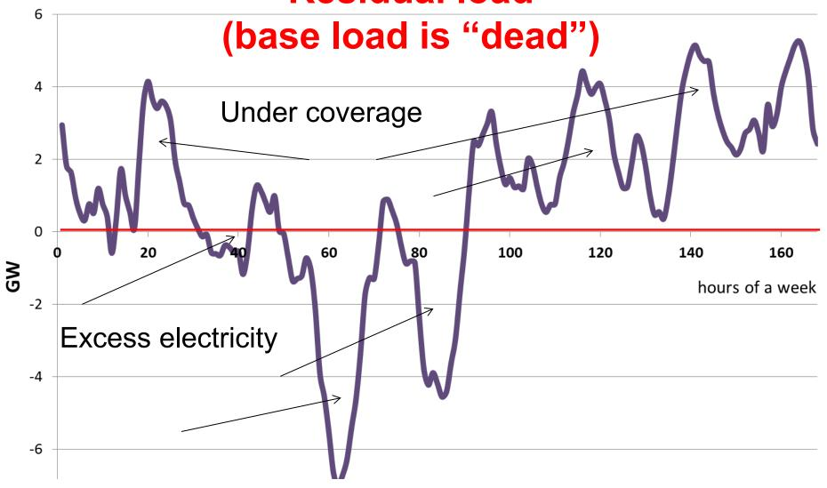
Residual load = Load - non-flexible generation
