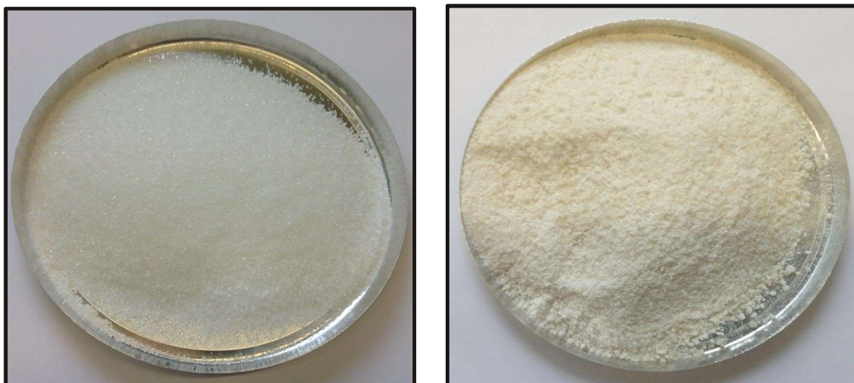
Figure 2.1.6 – Erythritol sample after (left) and before (right) 100 cycles under argon atmosphere
