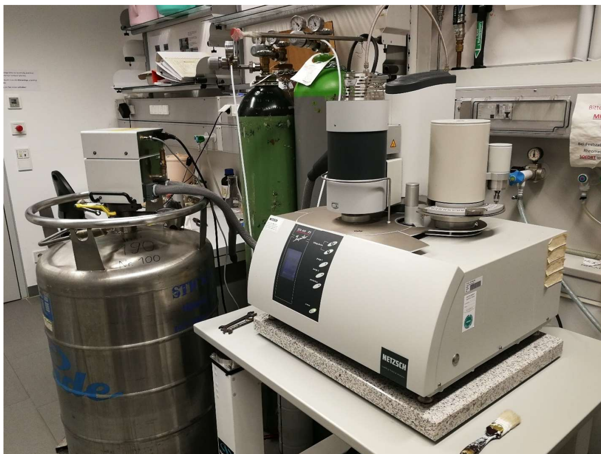
Figure 1.1.6 – STA 449 F1 JUPITER Netzsch employed in most of the STA measurement of this project
