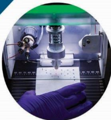
Direct Mass Analysis from TLC-plates – Plate Express™
