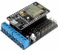
For the task, we've chosen the ESP8266 NodeMCU v.3 microcontroller as a cheap (less than 2 €) Wi-Fi ESP-12 based module. Together with the Motor Shield Board, based on L293D driver, it is sold for about 3.30 €.
