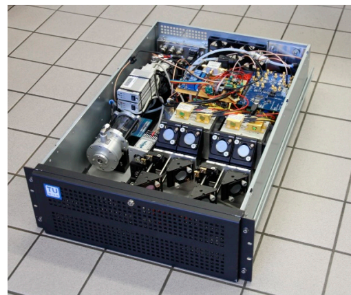
Figure 3. Schematic layout of the individual components for the 2f-WMS based sensor (a) and the assembly of the optical setup in a standard 19" server rack (b). The laser driver, data-acquisition-card, power supplies and the measurement PC are installed in a second rack (not shown).
