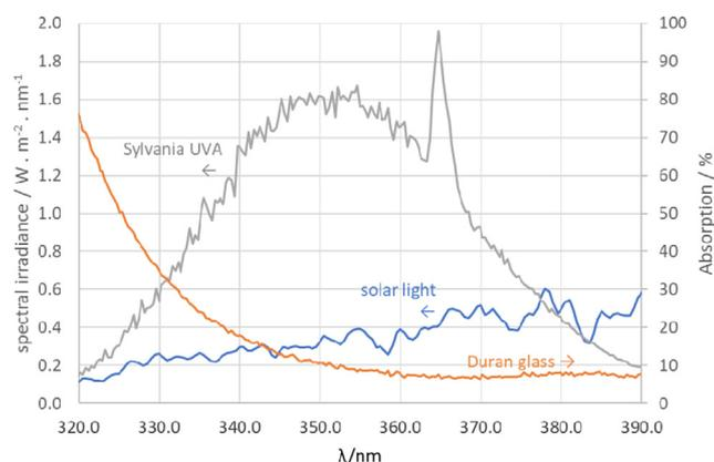
**Fig. 2.** Spectrum of UVA lamps, the absorption of Duran glass (thickness: 2 mm) and the solar spectrum (AM 1.5).
