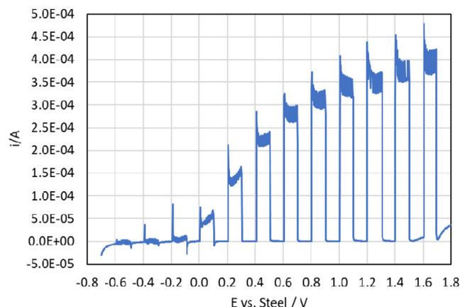
**Fig. 3.** Photoelectrochemical response of a TiO<sub>2</sub>/FTO electrode in buffered solution pH 10, under slow rectangular chopped UVA light.
