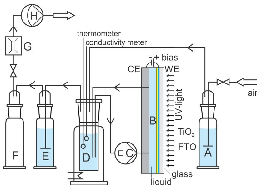
A. Absorption flask with fritted glass diffuser for CO<sub>2</sub> removal and H<sub>2</sub>O saturation, pH 14
