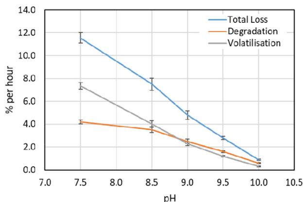
Fig. 4. Total and detailed cyanide loss in a degradation experiment, using 400 mg/l cyanide solutions in buffered solutions of different pH values. Initial loss values, in percent per hour.
