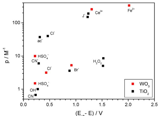
Fig. 5. Standardized rate constant – energy relationship. Constant  $p$  against the difference of the energy of the valence band to the redox potential of different species, using  $\text{WO}_3$  and  $\text{TiO}_2$  photocatalysts (data from Desilvestro and Graetzel, 1987; Frank and Bard, 1977; Hirano and Bard, 1980; Rappich and Dohrmann, 1990; Shinde et al., 2009; Kerchova et al., 1985).
