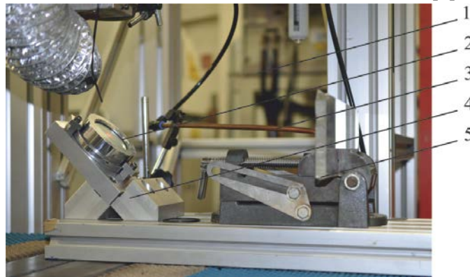
Figure 2. Photo of DOE as part of specific CO 2 laser equipment for metallic materials modification: 1 – CO 2 laser Oerlikon OPL 2000; 2 – DOE in the composition of the device, consisting of units for adjustment, fixation and cooling of the optical element; 3 – air supply hose; 4 – bedplate; 5 – means for measuring the power density distribution of laser beam.
