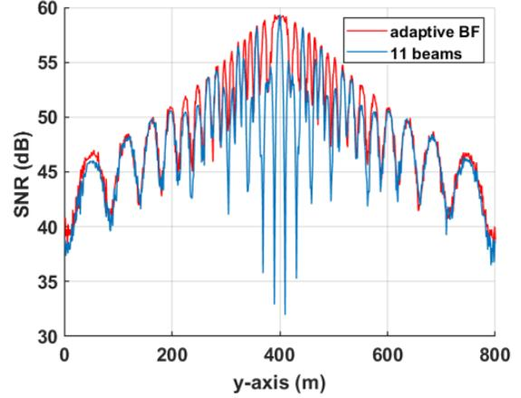
Fig. 2. SNR for adaptive BF and beam-switching with a horizontal ULA and 11 uniformly distributed fixed beams.
