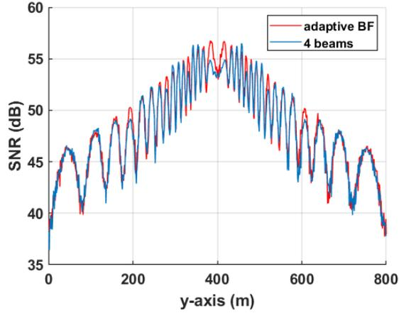
Fig. 4. SNR for adaptive BF and beam-switching with a vertical ULA and 4 uniformly distributed fixed beams.
