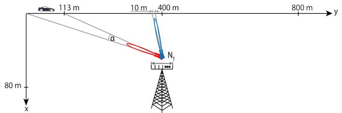
Fig. 1. An example beamwidth  $\alpha$  of 8.6 degree with a horizontally aligned ULA reaches two different lengths of the path depending on the steering angle.
