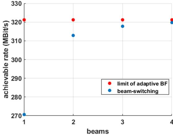
Fig. 5. Achievable rate for beam-switching with a vertical ULA compared to the limit from adaptive BF.
