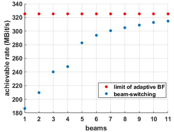
Fig. 3. Achievable rate for beam-switching with a horizontal ULA compared to the limit from adaptive BF.
