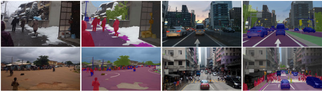
Figure 3.10: Example of diverse weather and lighting conditions with corresponding annotation data in Mapillary dataset. Original image in [NORBK17]
