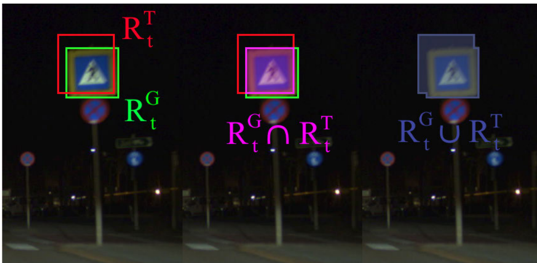
Figure 5.2: Visual explanation of IoU measure. Leftmost image shows ground truth ( R_t^G , green) and tracker's proposed region ( R_t^T , red), middle image shows region intersection ( R_t^G \cap R_t^T , magenta), and rightmost image shows union ( R_t^G \cup R_t^T , blue).
