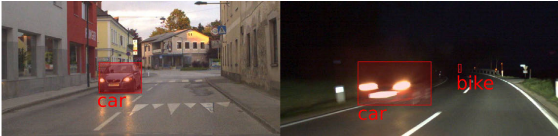
Figure 3.13: Day (left) and nighttime (right) example images from our CVL Dataset. Bigger red bounding boxes denoting oncoming vehicles, small bounding box in nighttime image denotes a bicycle and gives an example of how little visible information was recorded.
