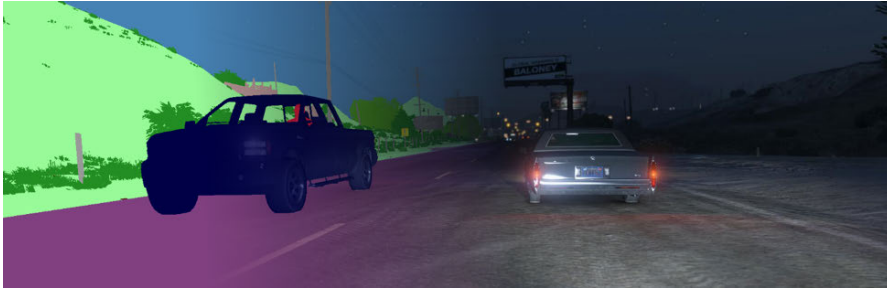
Figure 3.8: On the left side of this image we see the semantically segmentation mask overlaid and gradually faded out to one of the nighttime scenes from the VIPER dataset on the right.
