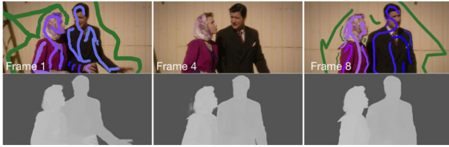
Figure 2.2: Example of nearly perfect 2D to 3D conversion using Brosch’s extended CVF technique. Original image in Brosch’s PhD Thesis [Bro16]
