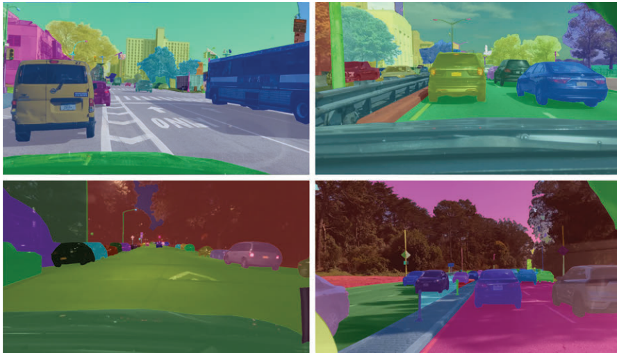
Figure 3.4: Example of fully segmented ground truth in BDD100k dataset. Original image in [YXC + 18].
