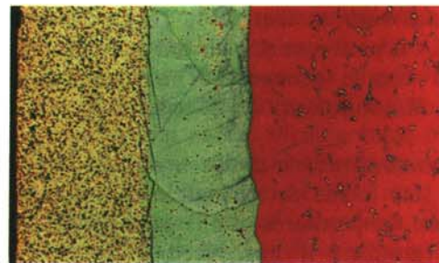
Fig. 6. Top: schematic diffusion profile in a three-phase diffusion couple. Bottom: corresponding microstructure. Nb–C couple: phase 3, \delta -NbC 1-x ; phase 2, \beta -Nb 2 C; phase 1, \alpha -Nb(C).
