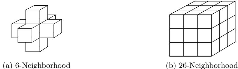
Figure 3.7: A scheme for the 6- and the 26-neighborhood of a voxel/element of a 3D matrix.
