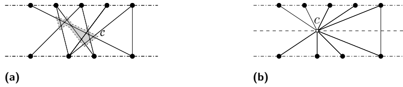
■ Figure 2 A crossing-patch in a graph that is not fan-planar, and how to contract it.
