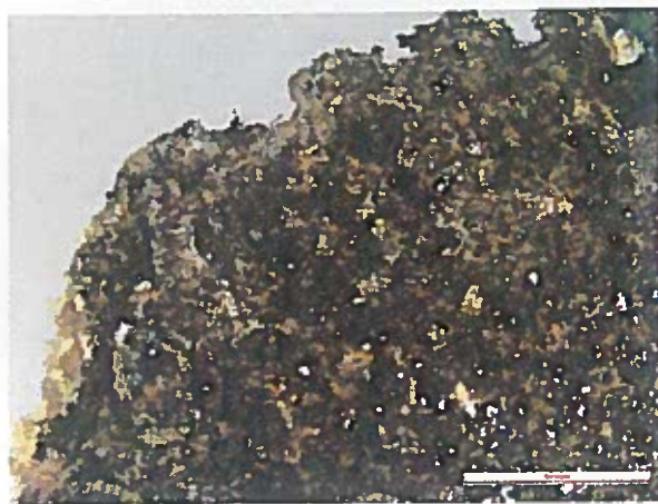
Figure 7: Black biogenic crust on Aflenz sandstone (scale-bar = 5 mm).
