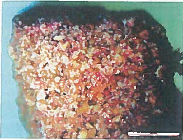
Figure 6: PAS stain of St. Margarethen sandstone (scale-bar = 5 mm).
